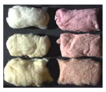
The importance of Average Colour to the Dyer is illustrated opposite. The left of the picture shows three samples of scoured and carded wool, where the yellowness increases progressively.
